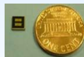
Sensor chip with gold electrode pads and active polymer region for sensing application.
